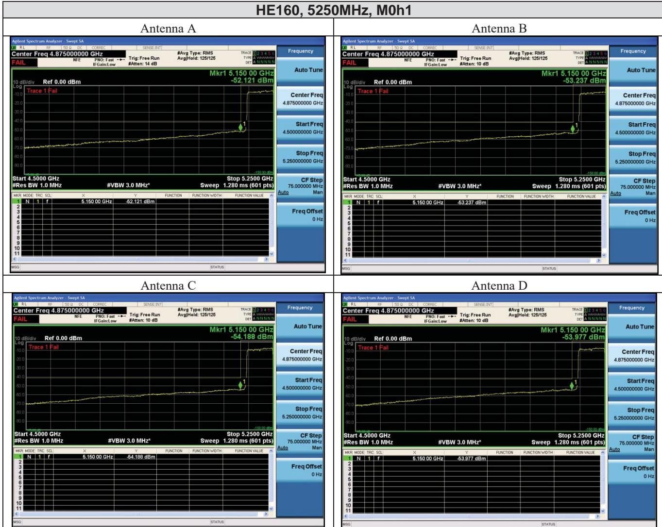
Note: Traces say fail above because the transmitter is above an arbitrary line in the pass band
