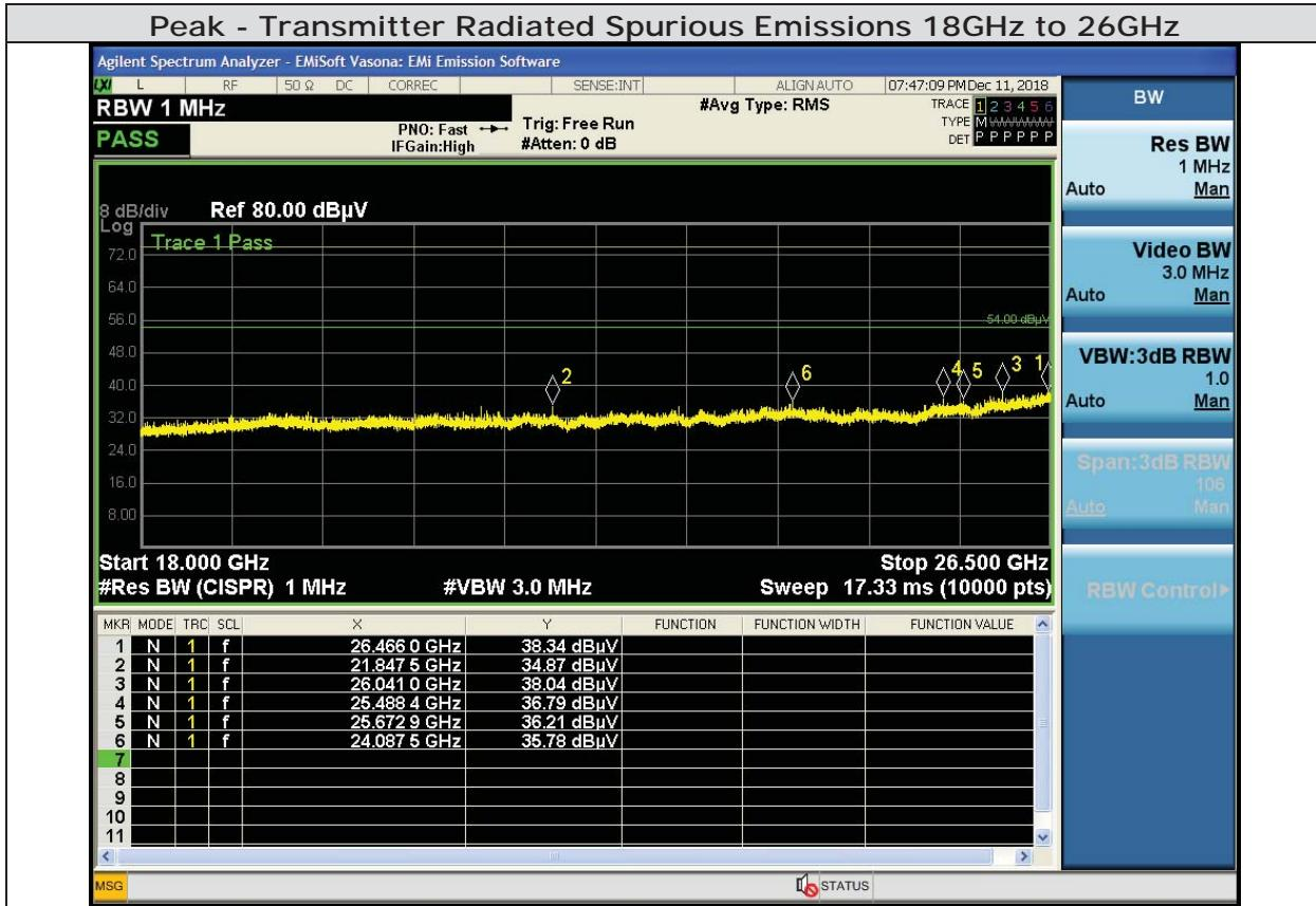
Note: Emissions tests were done with all radios on simultaneously (i.e. BLE, 2.4GHz, and 5GHz radios). EUT is in worst case mode
