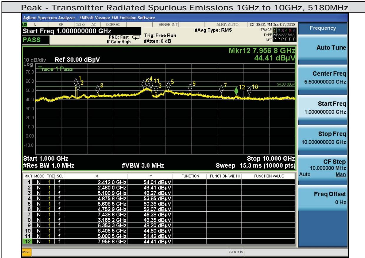
Note: Emissions tests were done with all radios on simultaneously (i.e. BLE, 2.4GHz, and 5GHz radios)
