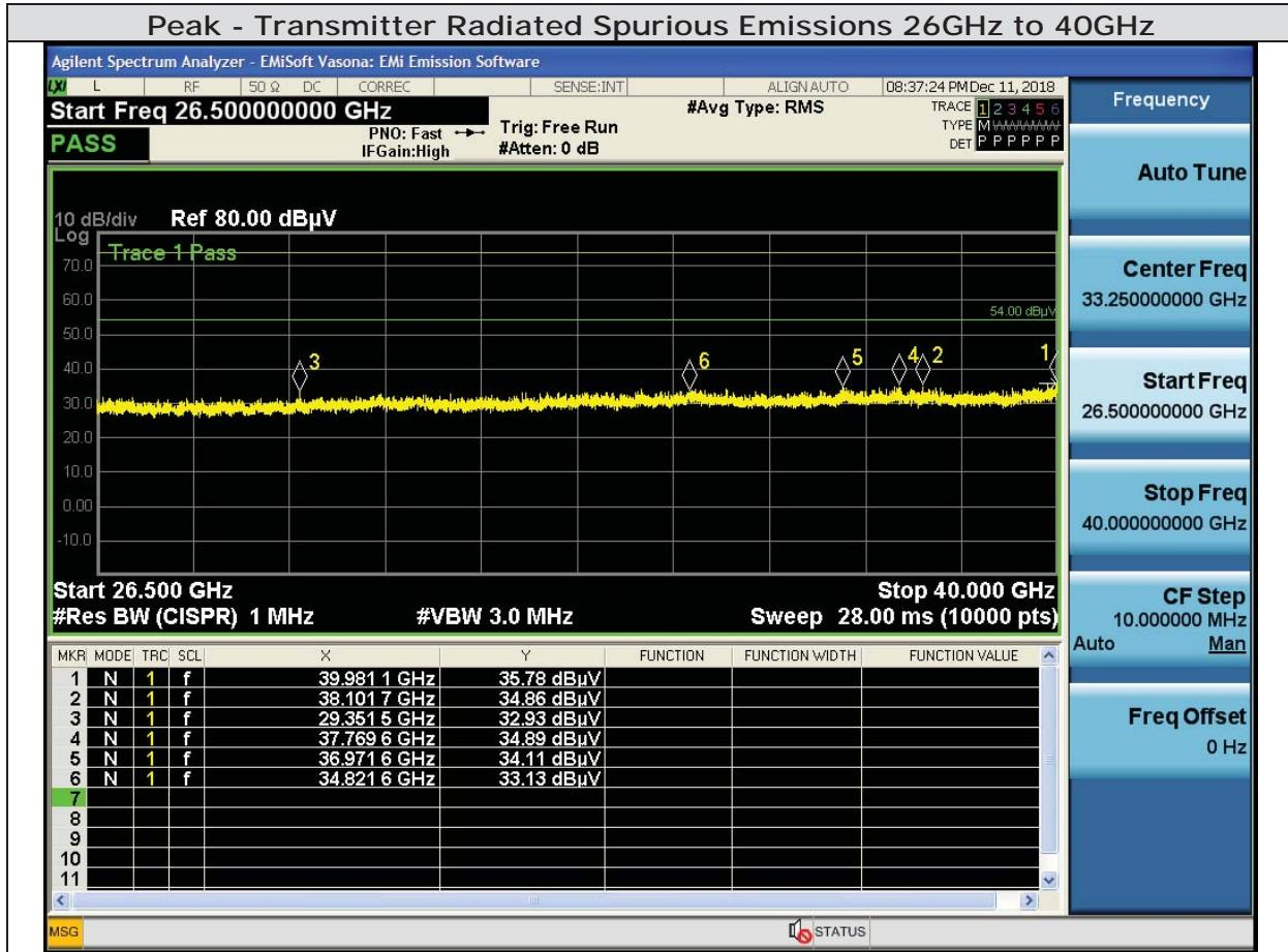
Note: Emissions tests were done with all radios on simultaneously (i.e. BLE, 2.4GHz, and 5GHz radios). EUT is in worst case mode
