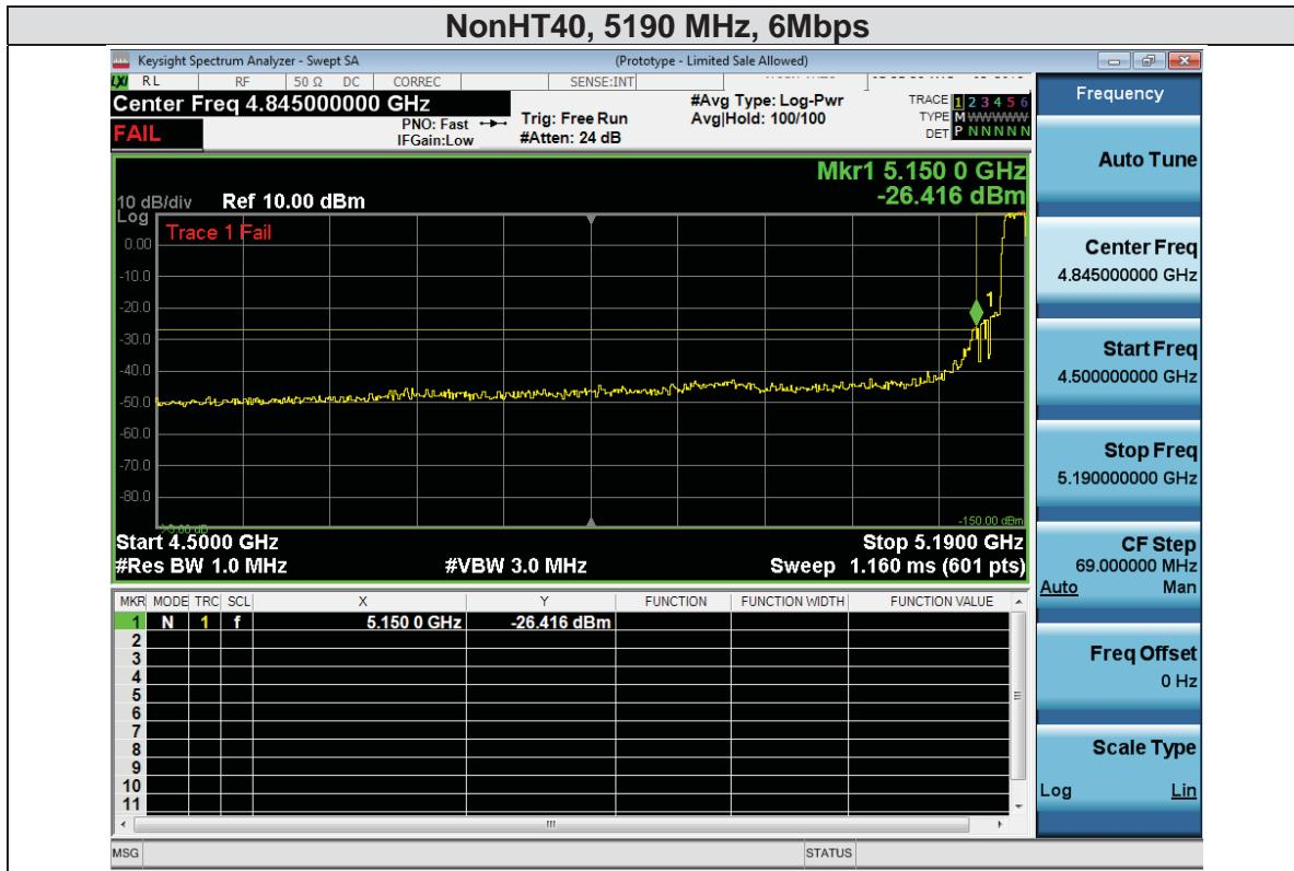
Note: Traces say fail above because the transmitter is above an arbitrary line in the pass band
