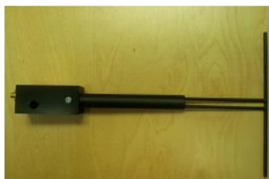
Figure 1 – MVG COMOSAR Validation Dipole
