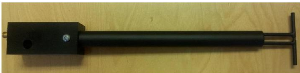
Figure 1 – MVG COMOSAR Validation Dipole
