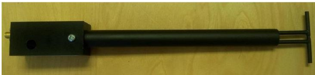
Figure 1 – MVG COMOSAR Validation Dipole
