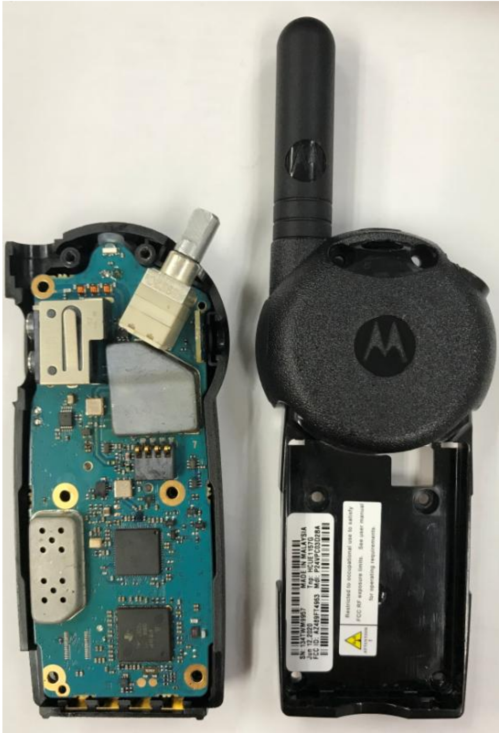
RF board with chassis and housing (Back Side) [VL50: P24VPC03D2BA]
