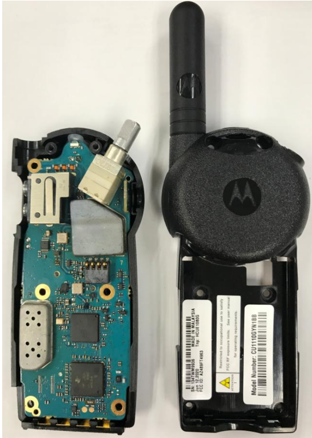
RF board with chassis and housing (Back Side) [CLS1110: CU110GYN1BB]
