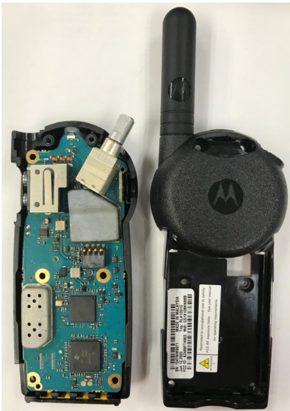
RF board with chassis and housing (Back Side) [CLS1810T: GS1810BKN8BB]
