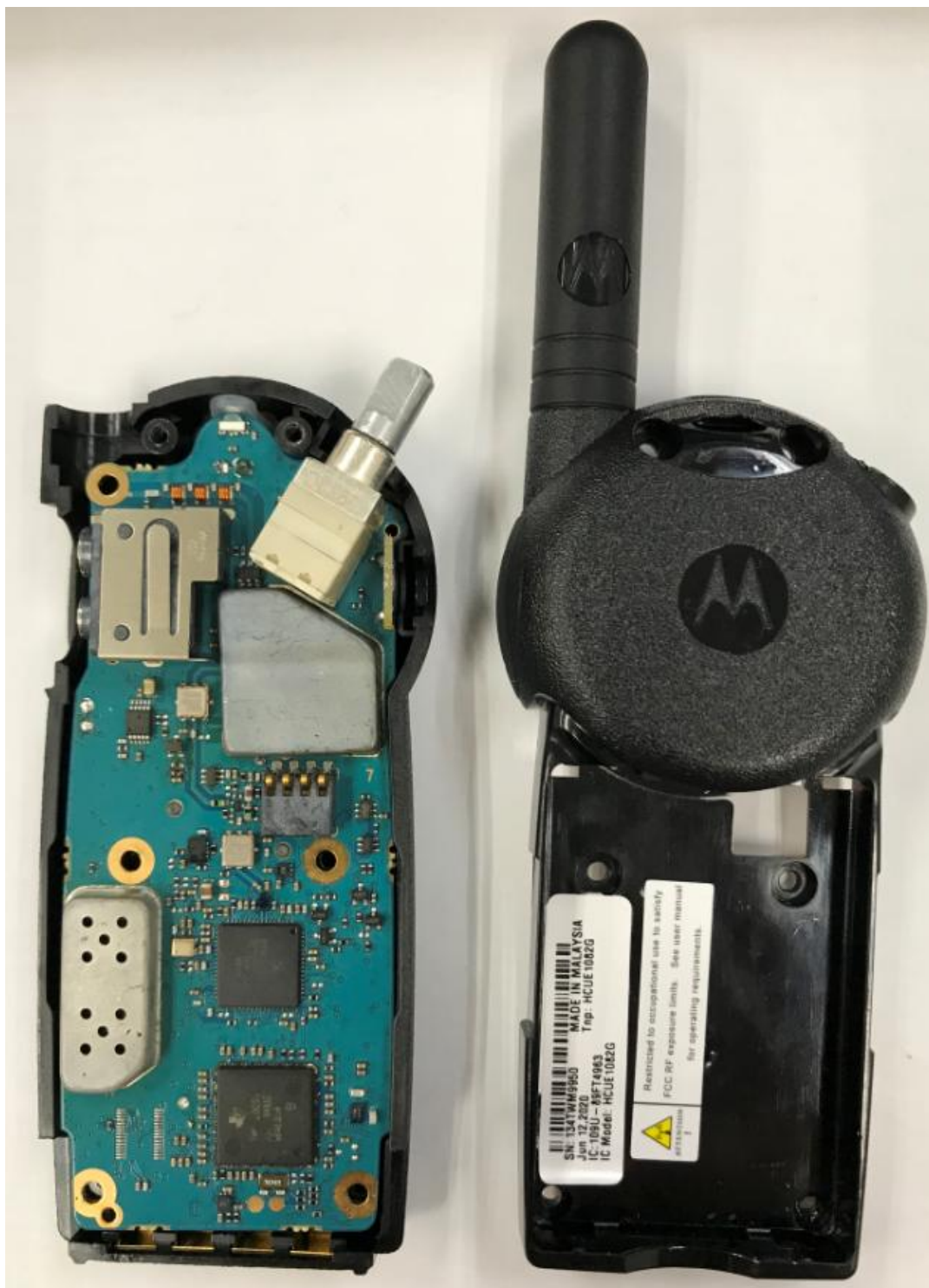
RF board with chassis and housing (Back Side) [CLS1413: HCUE1082G]
