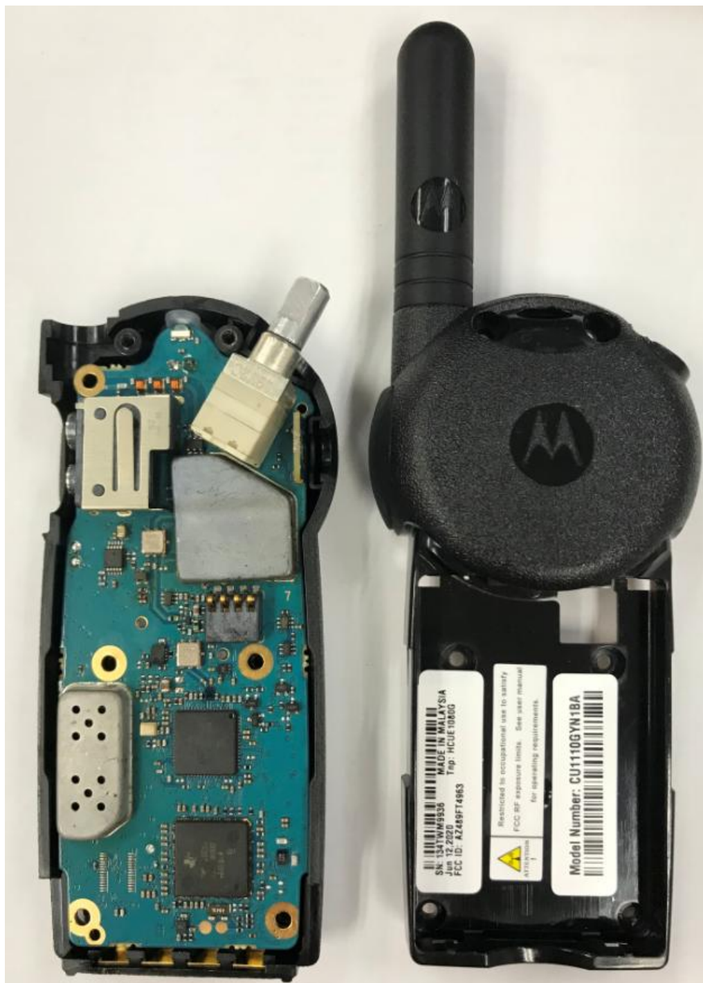
RF board with chassis and housing (Back Side) [CLS1110: CU1110GYN1BA]
