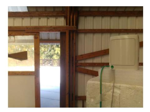
Photograph No.11 Spurious emissions measurement setup at the OATS above 40 GHz, 0.05 m test distance
