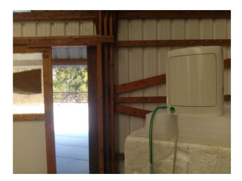
Photograph No.10 Spurious emissions measurement setup at the OATS above 40 GHz, 0.5 m test distance
