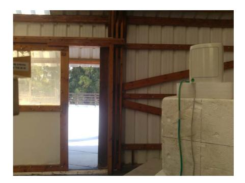
${\bf Photograph~No.9}\\ {\bf Spurious~emissions~measurement~setup~at~the~OATS~above~40~GHz,~0.5~m~test~distance}\\$
