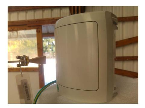
Photograph No.12 Spurious emissions measurement setup at the OATS above 40 GHz, 0.01 m test distance
