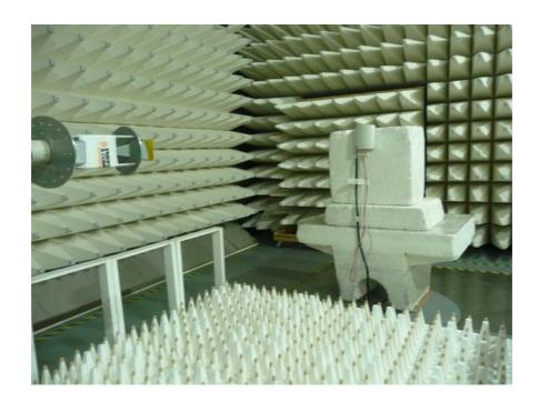
Photograph No.7 Spurious emissions measurement setup at the OATS above 40 GHz, 3 m test distance
