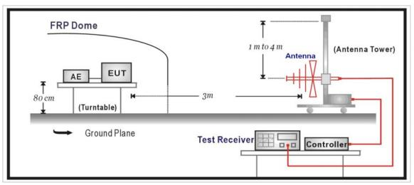
Above 1GHz Test Setup:
