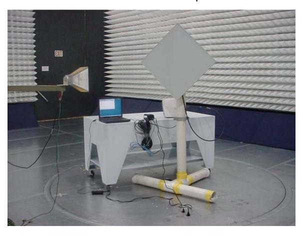
FCC ID: HZB-S58-S60C Radiated Emissions Test Setup
