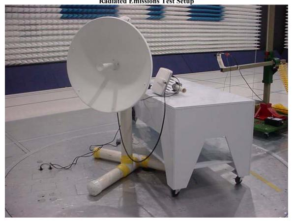
FCC ID: HZB-S58-S60C Radiated Emissions Test Setup
