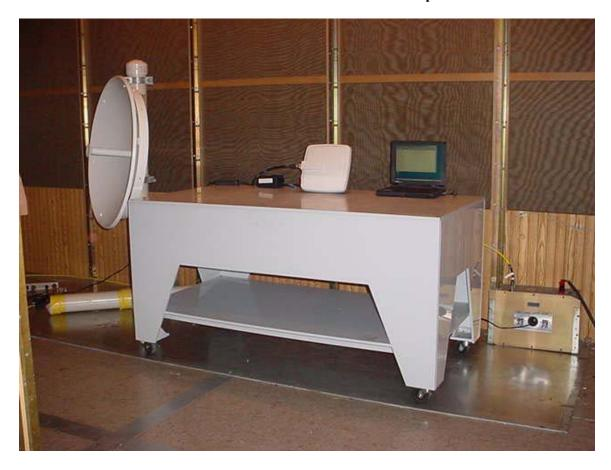
FCC ID: HZB-S58-S60C AC line-conducted Emissions Test Setup
