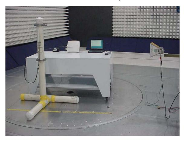
FCC ID: HZB-S58-S60C Radiated Emissions Test Setup
