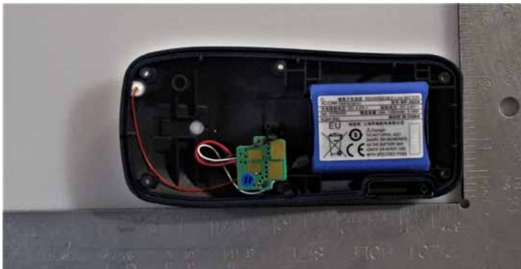
<Li-ion Chargeable Battery (BP-282N, 3.6V, 1570mAh)>
