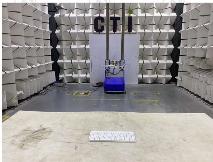
Radiated spurious emission Test Setup-1(Below 1GHz)
