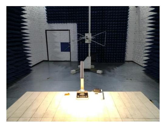
FCC RADIATED EMISSION TEST SETUP ABOVE 1GHZ
