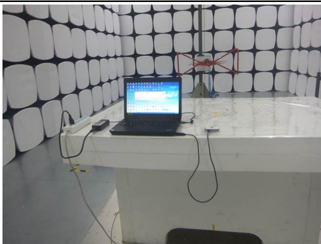
Conducted Emissions Test Setup Front View
