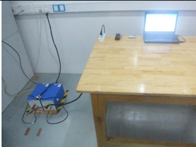
Conducted Emissions Test Setup Front View
