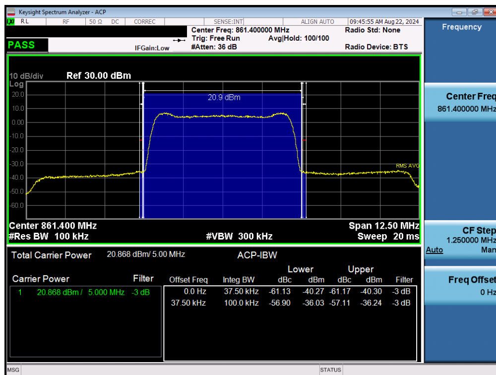
Plot 7-10. Channel Edge Plot – Low Channel (UMTS Band 26 - 5MHz)
