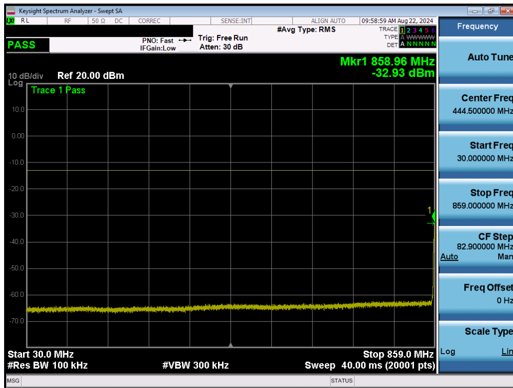
Plot 7-4. Conducted Spurious Plot – Low Channel (UMTS Band 26 - 5MHz)
