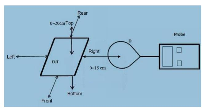
Note: Measurements should be made from all sides and the top of the primary/client pair, with the 20 cm-0cm measured from the center of the top, and 15cm-0cm measured from the center of the rest
