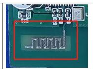
The antenna is PCB antenna.
