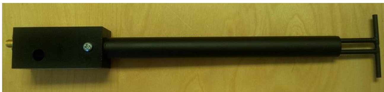
Figure 1 – MVG COMOSAR Validation Dipole
