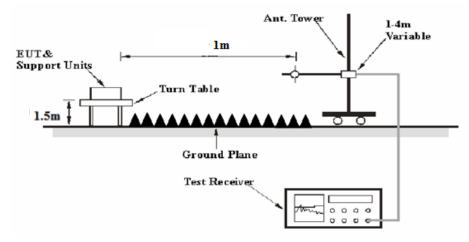
The radiated emission Below 1GHz tests were performed in the 10 meters chamber test site, above 1GHz tests were performed in the 3 meters chamber test site B, using the setup accordance with the ANSI C63.10-2013. The specification used was the FCC 15.209, and FCC 15.407 limits and RSS-247, RSS-Gen limits.
