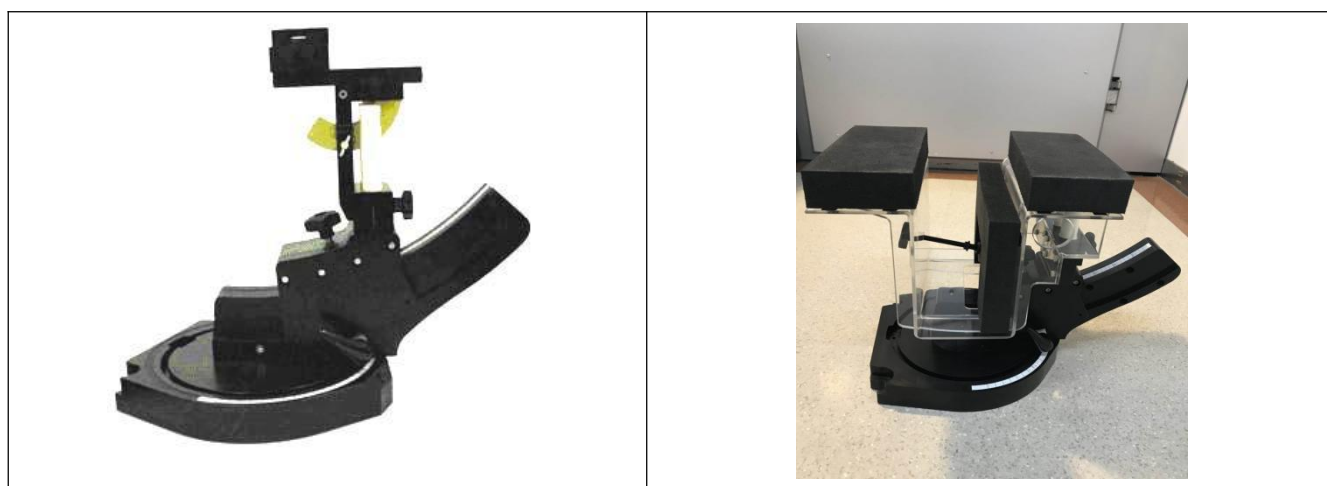
Device holder supplied by SPEAG
