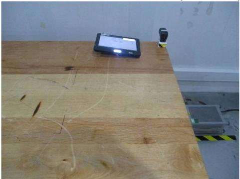
1.2 Radiated Emissions (9kHz-30MHz) Test Setup
