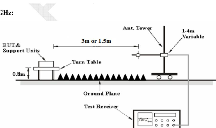
The radiated emission tests were performed in the 3 meters chamber, using the setup accordance with the ANSI C63.4-2009. The specification used was the FCC 15.209, and FCC 15.407 limits.
