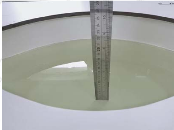
Liquid depth in the body phantom (2450MHz)
