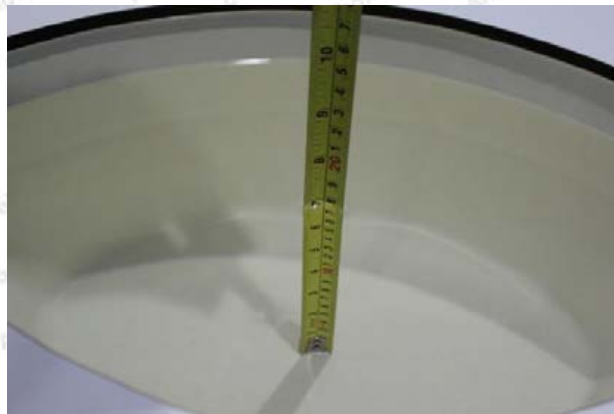
Liquid depth in the body phantom (5GHz)
