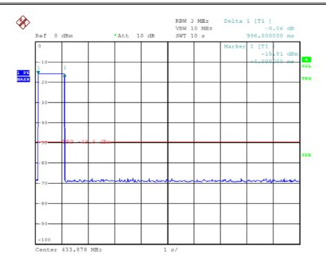
Result: After pushing the handle of EUT, emission was found to cease within 5 seconds.
