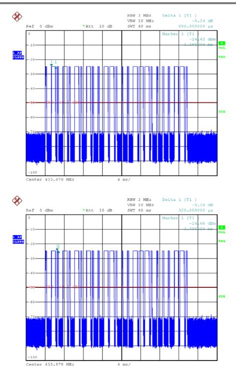
Timing Plot – Pursuant to FCC Part 15 Section 15.231(a)
