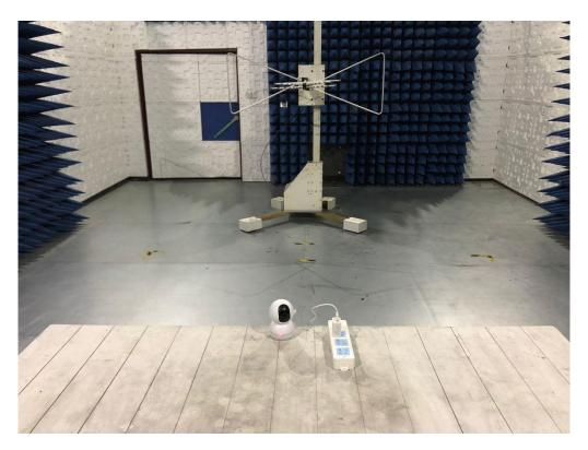
FCC RADIATED EMISSION TEST SETUP ABOVE 1GHZ
