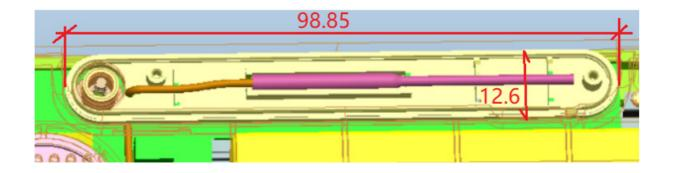
Figure 1 Physical dimension (mm)
