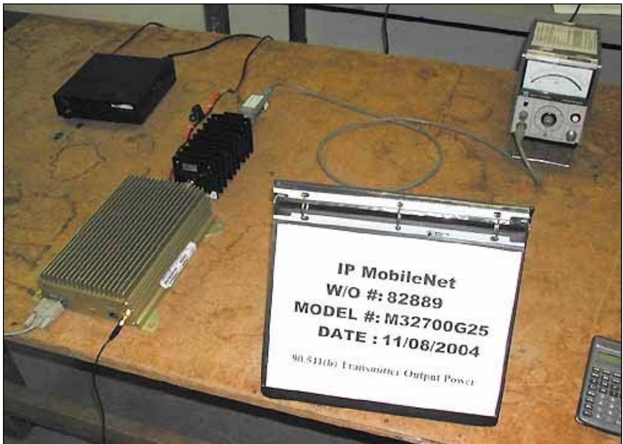
PHOTOGRAPH SHOWING TRANSMITTER OUTPUT POWER
