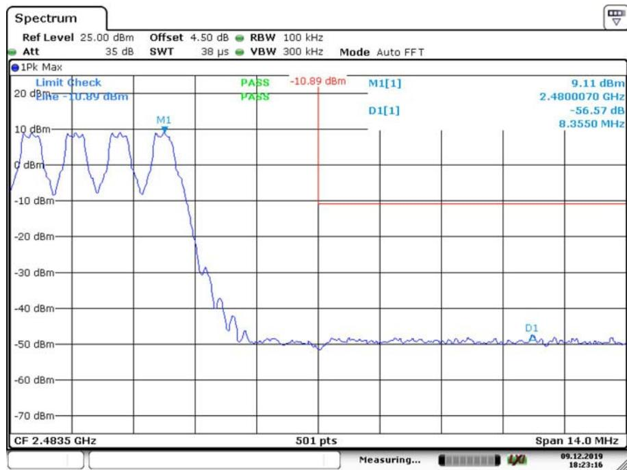
*EDR Mode ( $\pi/4$ -DQPSK):***Band Edge, Left Side**
