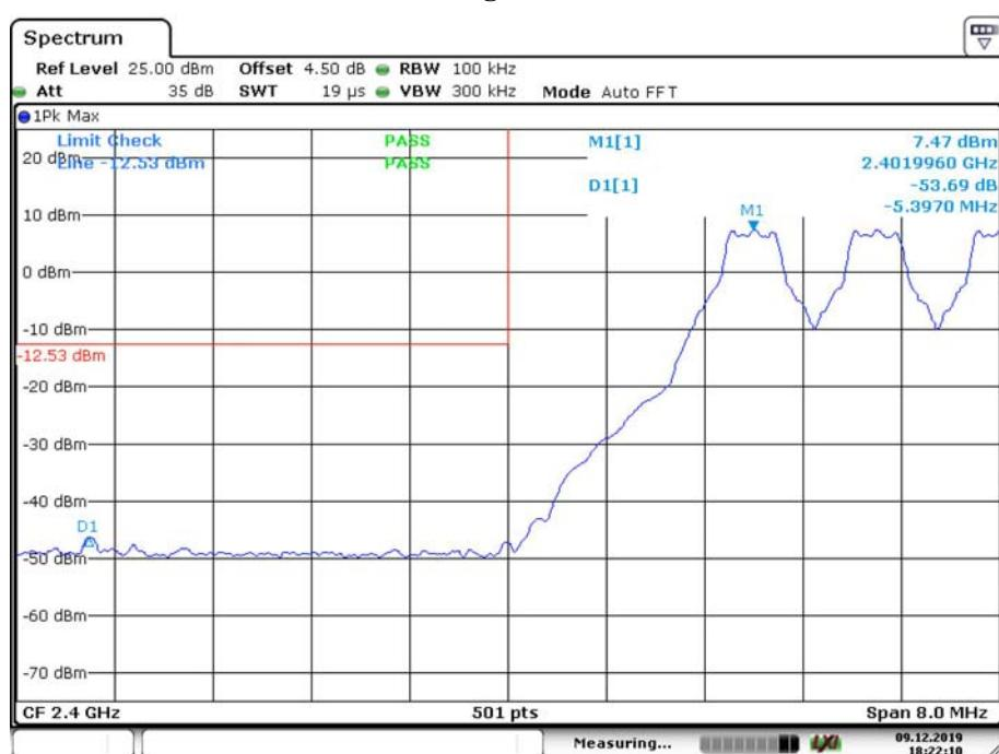
**Band Edge, Right Side**
