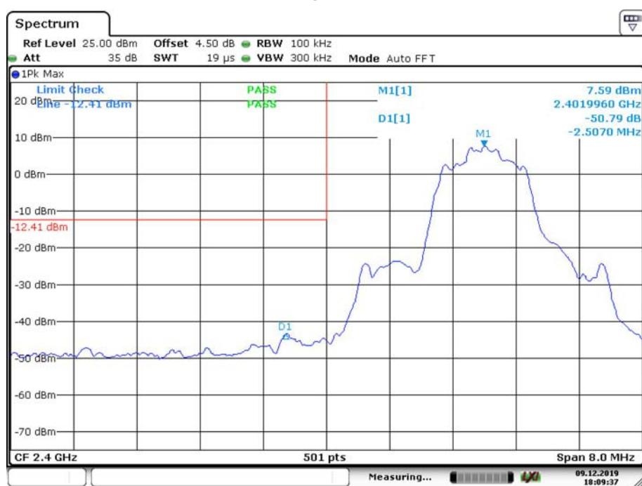
**Band Edge, Right Side**
