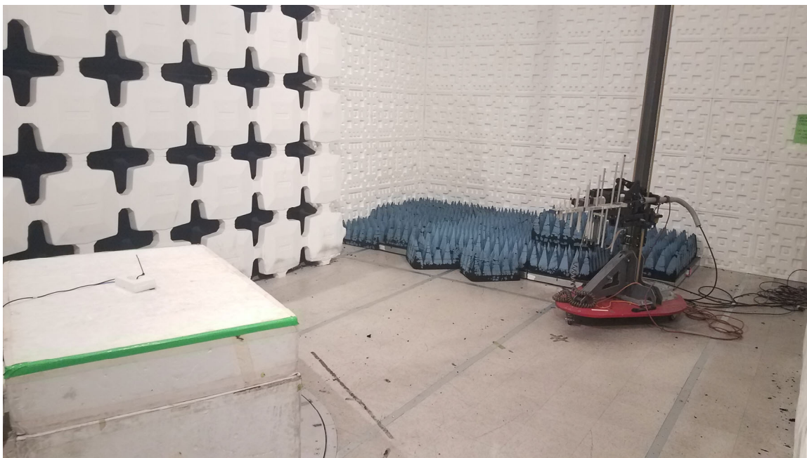
Figure 4. Radiated Emissions Test Setup, 200 MHz to 1000 MHz
