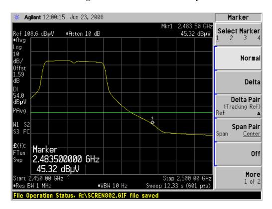
Detector mode: Peak Polarity: Horizontal
