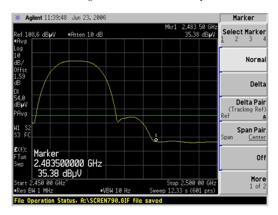
Detector mode: Peak Polarity: Horizontal
