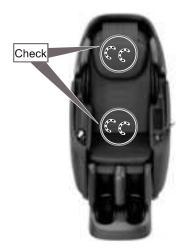
If rollers are not positioned correctly at the top of the backrest and at the waist of the backrest, press the power button to reset them to the default position.
