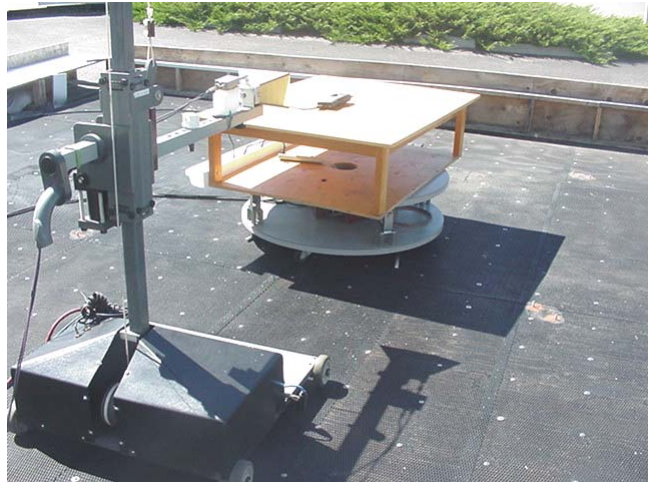
Photograph D.7-2 - Horn Receive Antenna with IX100X and MaxRad Vehicle-Mount Antenna Configuration
