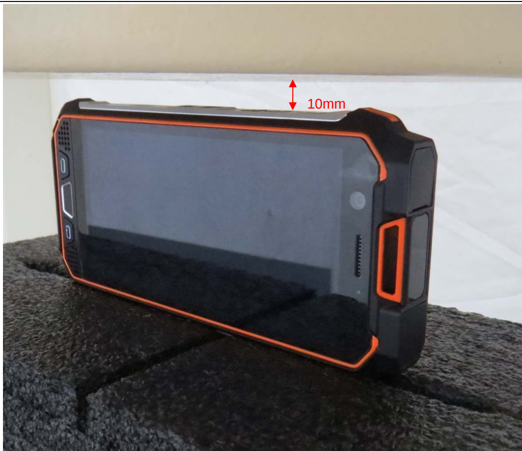
Picture 9: Left Side, the distance from handset to the bottom of the Phantom is 10mm
