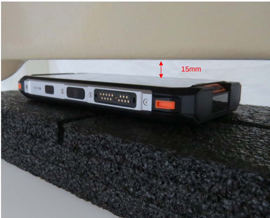
Picture 6: Front Side, the distance from handset to the bottom of the Phantom is 15mm
