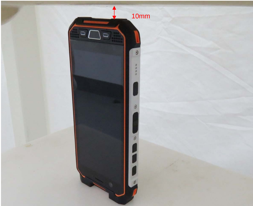
Picture 12: Bottom Edge, the distance from handset to the bottom of the Phantom is 10mm
