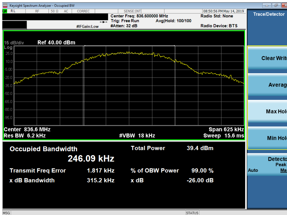
Plot 7-1. Occupied Bandwidth Plot (Cellular GPRS Mode)
