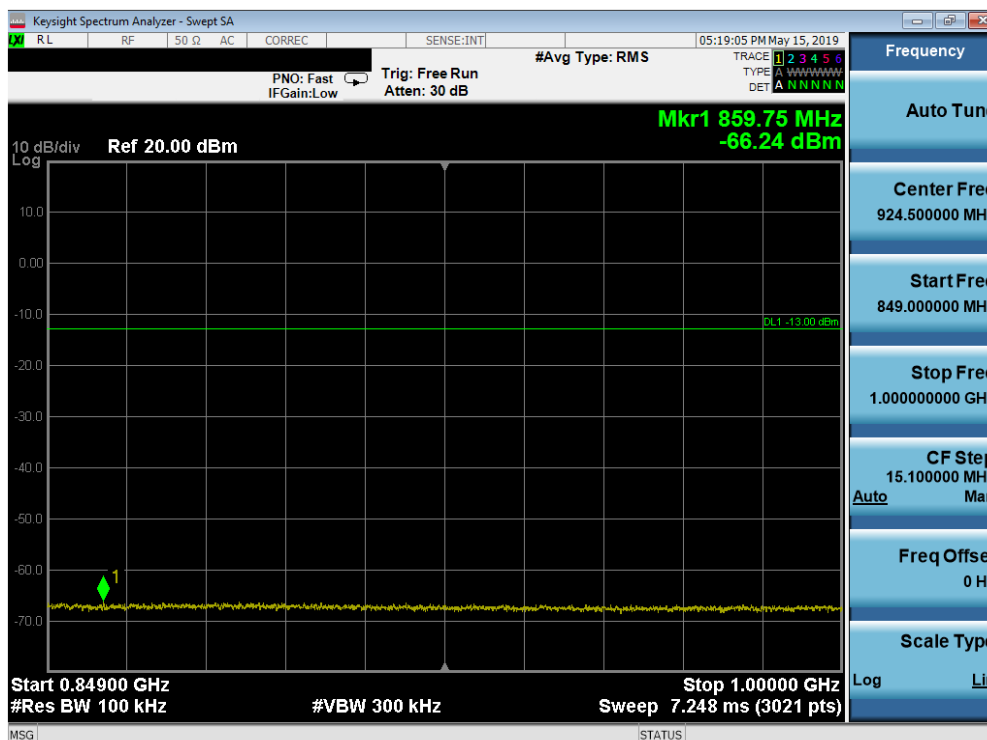
Plot 7-29. Conducted Spurious Plot (Cellular CDMA Mode - Low Channel)
