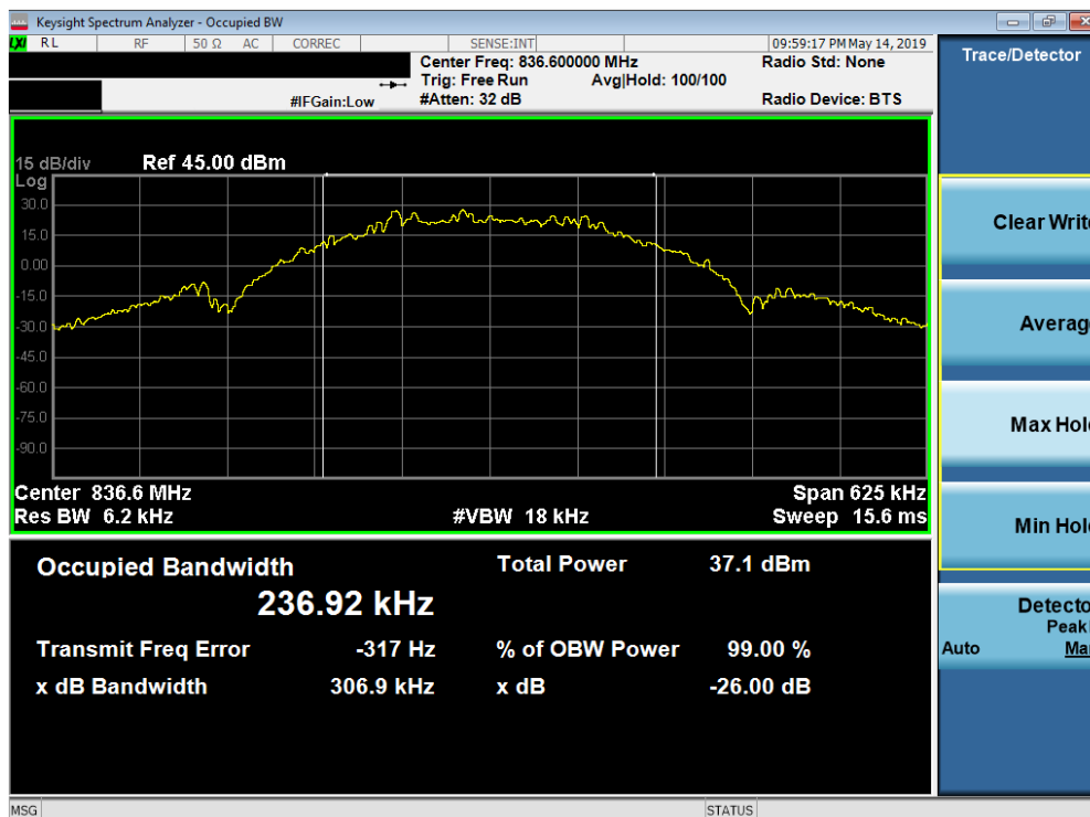
Plot 7-2. Occupied Bandwidth Plot (EDGE850 Mode)
