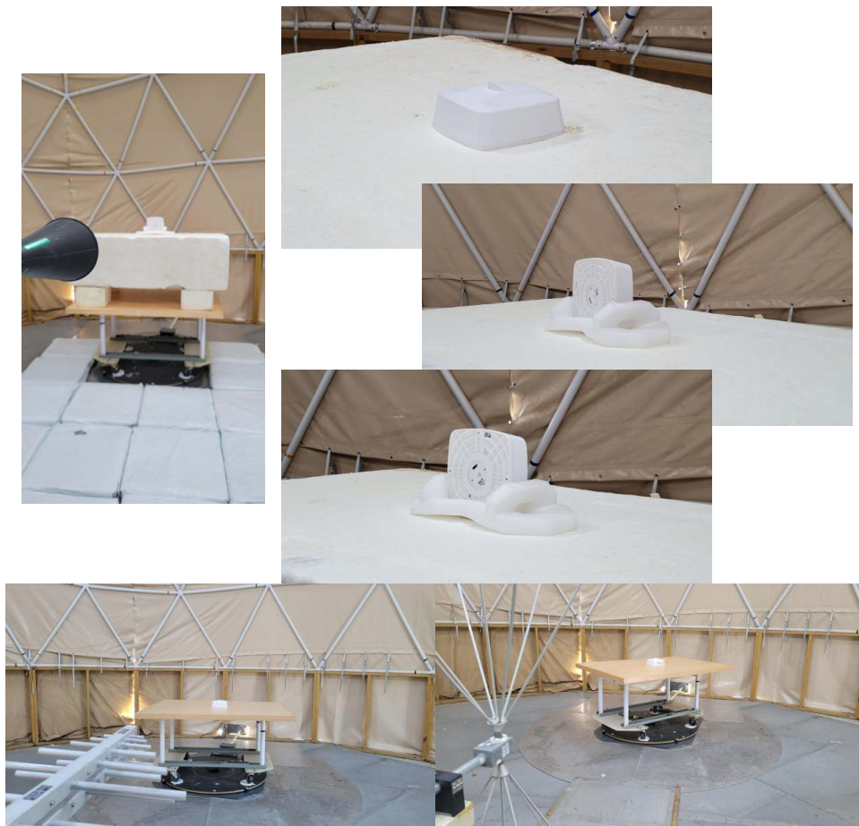
Figure 4.1.1 Radiated Emissions Test Setup Photograph(s).
