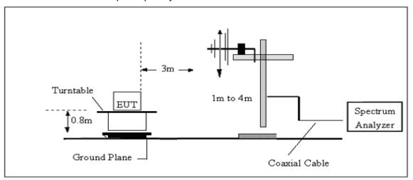
3. Radiated Emission Test-Up Frequency Above 1GHz
