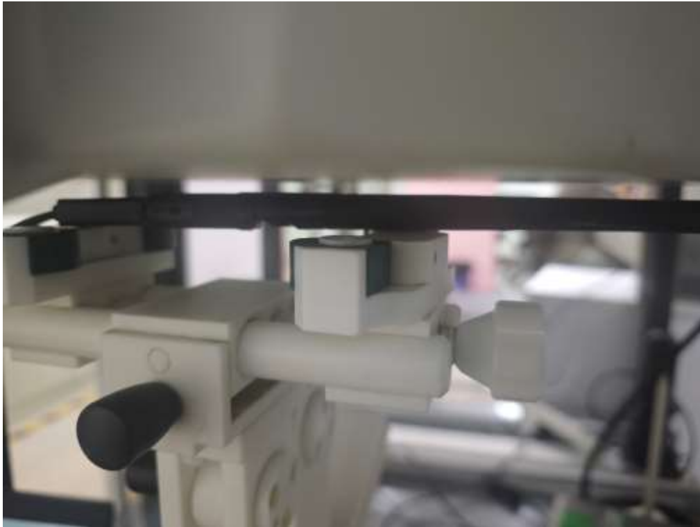
Model Name: WD-AX903 Horizontal- Up Antenna straight (separation distance is 5mm)
