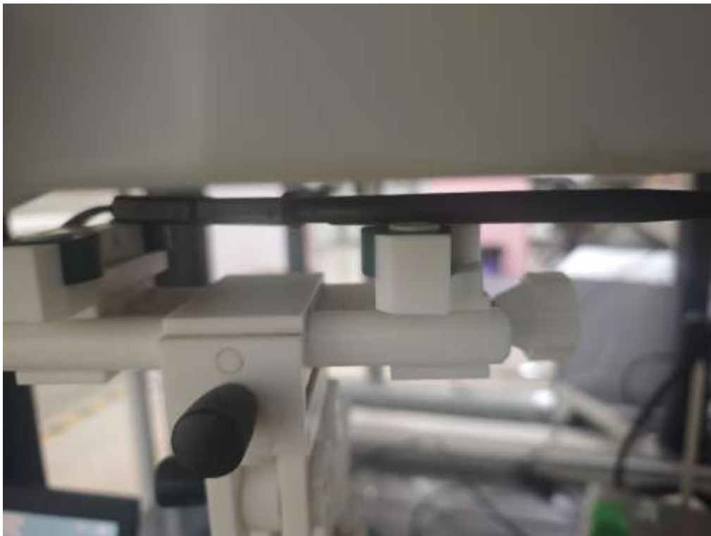
Model Name: WD-AX906 Horizontal- Down Antenna straight (separation distance is 5mm)
