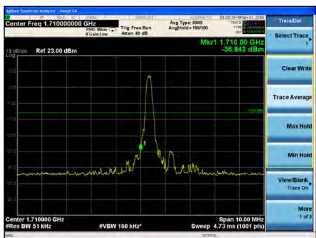
LTE Band 4 16QAM 5MHz CH-Low, 100%RB
