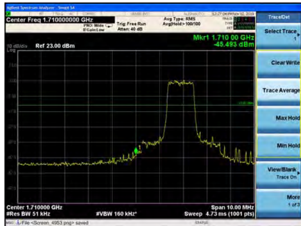
LTE Band 66 16QAM 1.4MHz CH-Low, 1 RB
