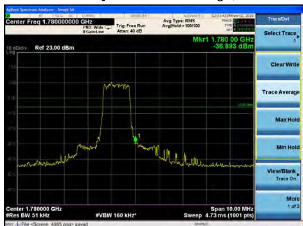
LTE Band 66 QPSK 10MHz CH-High, 1 RB
