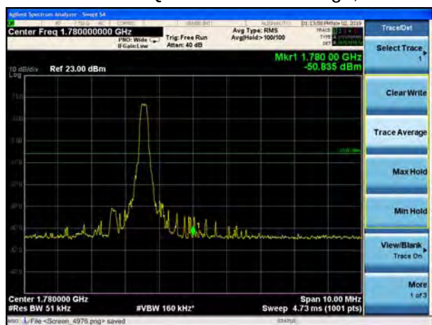
LTE Band 66 QPSK 20MHz CH-High, 1 RB
