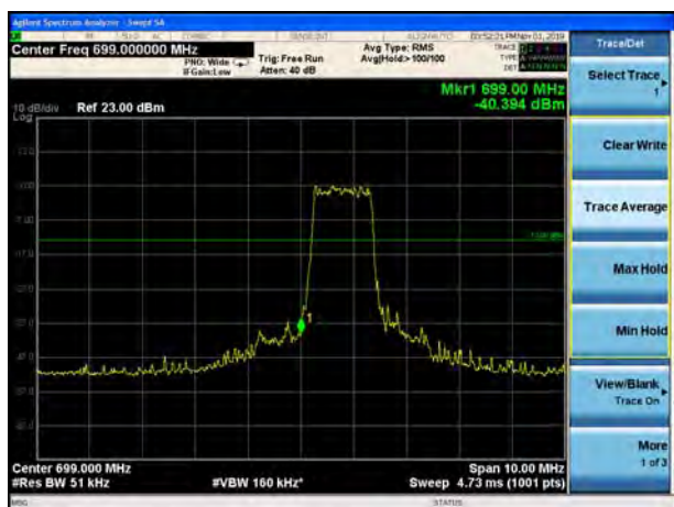
LTE Band 12 QPSK 5MHz CH-Low, 100%RB
