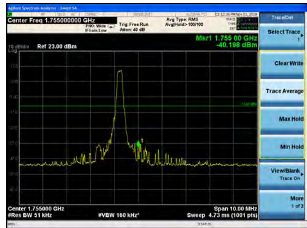
LTE Band 4 QPSK 10MHz CH-High, 100%RB
