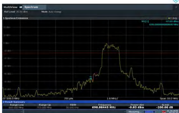
LTE Band 85 16QAM 10MHz CH-Low, 100%RB
