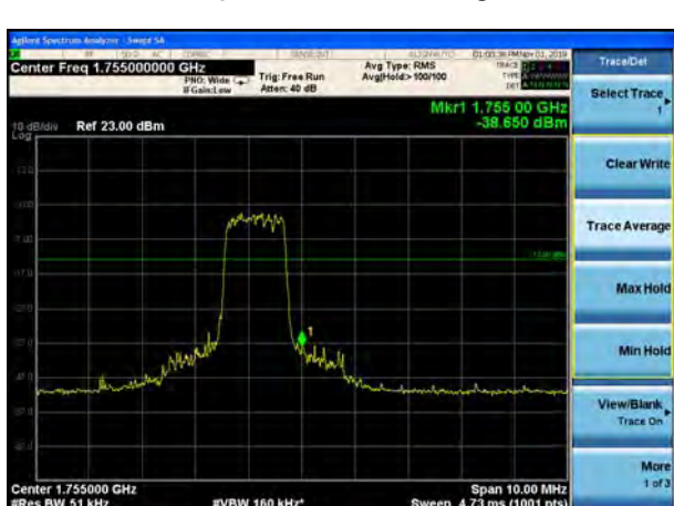
LTE Band 4 QPSK 3MHz CH-High, 100%RB
