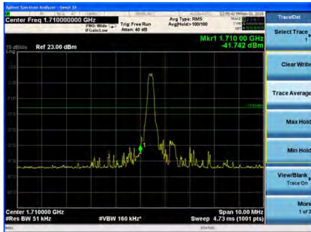
LTE Band 4 16QAM 3MHz CH-Low, 1 RB
