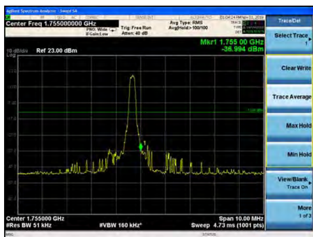
LTE Band 4 16QAM 5MHz CH-High, 100%RB
