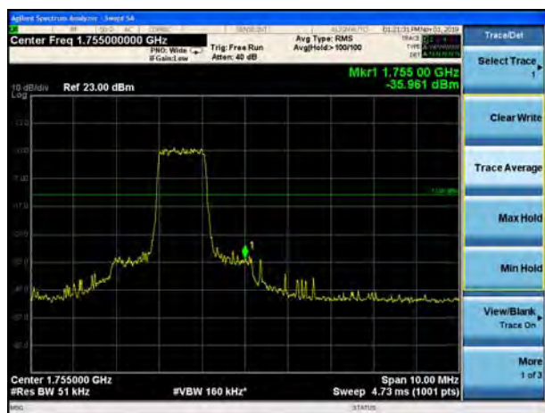
LTE Band 4 QPSK 20MHz CH-High, 1 RB
