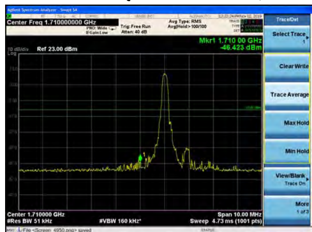
LTE Band 66 16QAM 15MHz CH-Low, 100%RB
