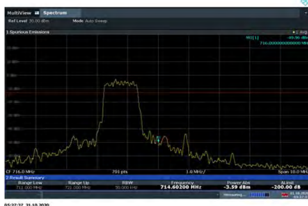
LTE Band 85 16QAM 5MHz CH-High, 1 RB
