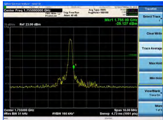
LTE Band 4 16QAM 1.4MHz CH-High, 100%RB
