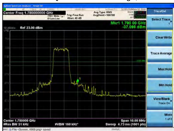
LTE Band 66 QPSK 10MHz CH-High, 100%RB
