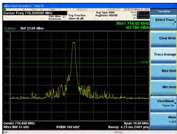
LTE Band 12 QPSK 3MHz CH-High, 1 RB
