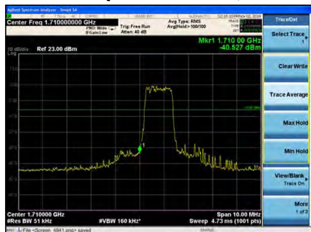
LTE Band 66 QPSK 10MHz CH-Low, 1 RB
