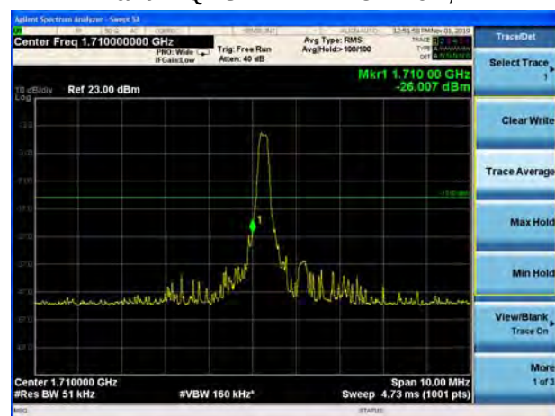
LTE Band 4 QPSK 1.4MHz CH-Low, 100%RB
