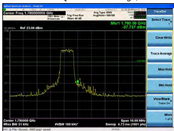
LTE Band 66 16QAM 5MHz CH-High, 1 RB
