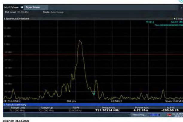
LTE Band 85 QPSK 10MHz CH-High, 100%RB
