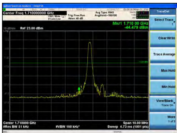
LTE Band 4 16QAM 10MHz CH-Low, 100%RB
