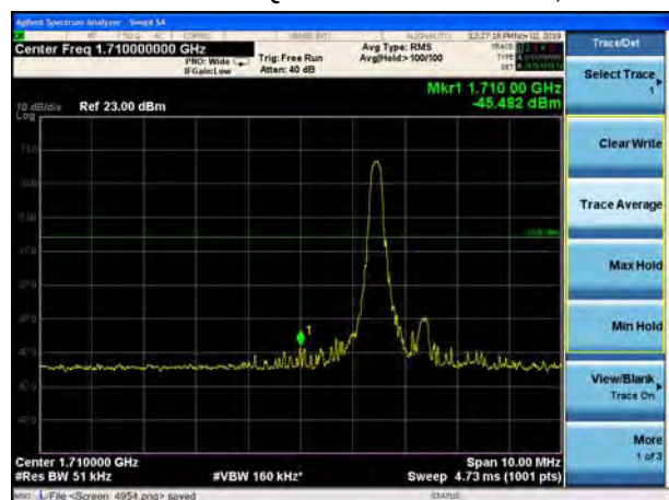
LTE Band 66 16QAM 20MHz CH-Low, 1 RB
