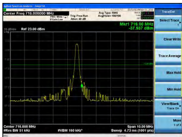
LTE Band 12 16QAM 5MHz CH-High, 100%RB
