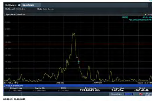
LTE Band 85 QPSK 5MHz CH-High, 100%RB
