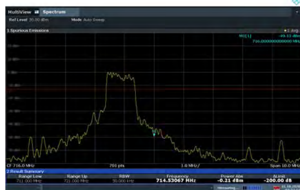
LTE Band 85 16QAM 10MHz CH-High, 100%RB
