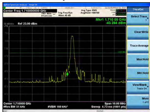
LTE Band 66 16QAM 3MHz CH-Low, 100%RB
