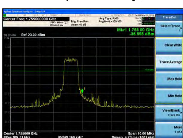
LTE Band 4 16QAM 3MHz CH-High, 100%RB
