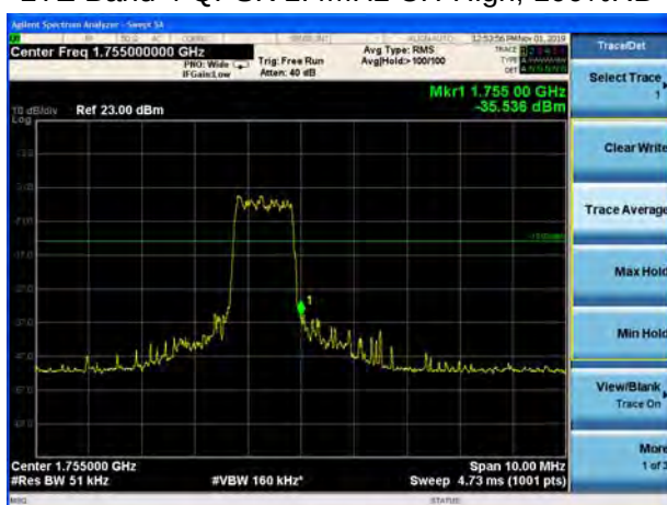
LTE Band 4 QPSK 3MHz CH-High, 1 RB
