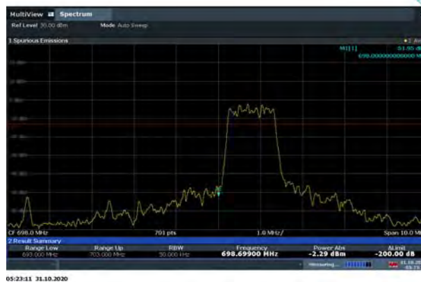
LTE Band 85 QPSK 5MHz CH-Low, 100%RB
