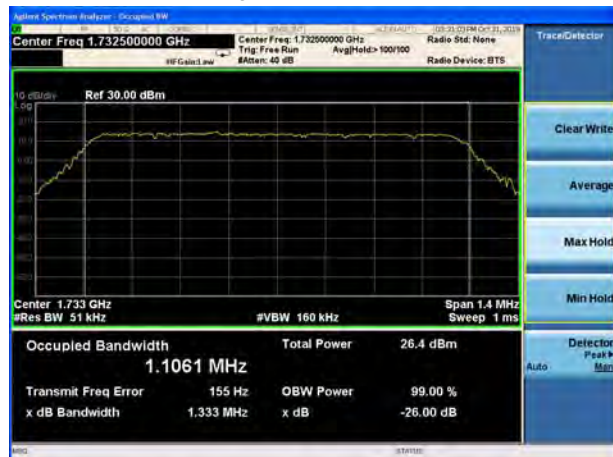
LTE Band 4 QPSK 5MHz CH-Middle
