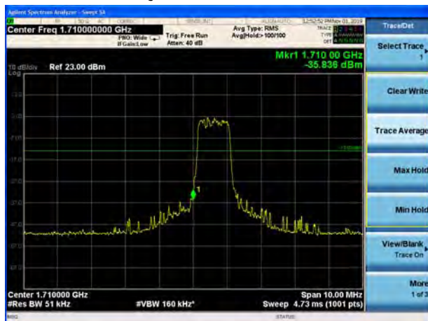
LTE Band 4 16QAM 3MHz CH-Low, 1 RB
