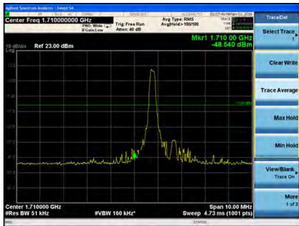
LTE Band 4 QPSK 10MHz CH-Low, 100%RB
