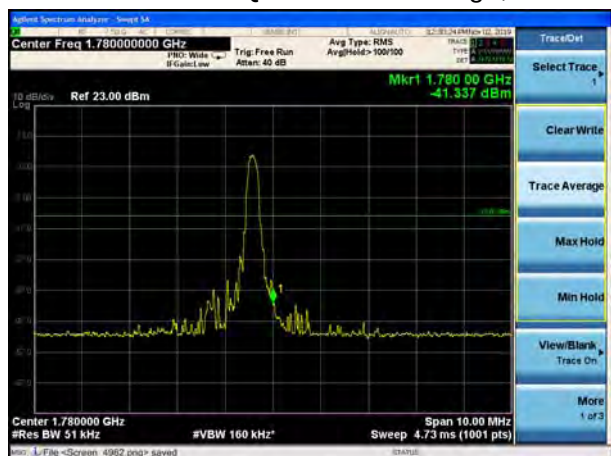
LTE Band 66 16QAM 3MHz CH-High, 100%RB
