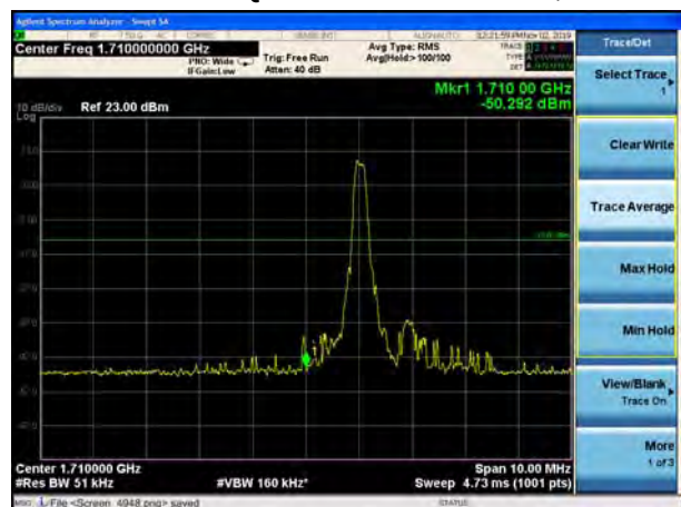
LTE Band 66 QPSK 15MHz CH-Low, 100%RB
