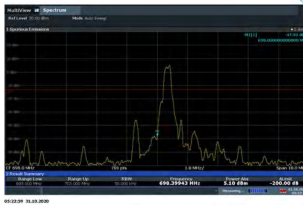
LTE Band 85 QPSK 5MHz CH-Low, 100%RB
