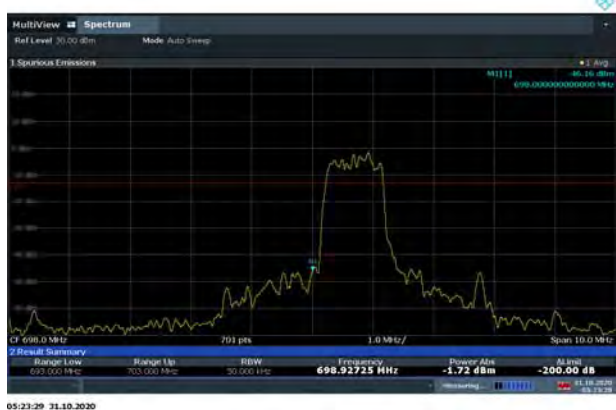
LTE Band 85 16QAM 10MHz CH-Low, 1 RB
