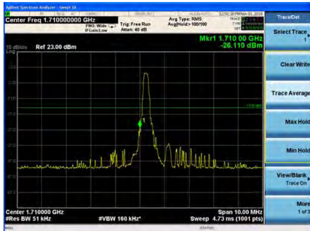
LTE Band 4 16QAM 1.4MHz CH-Low, 100%RB
