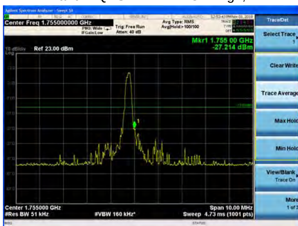
LTE Band 4 QPSK 1.4MHz CH-High, 100%RB
