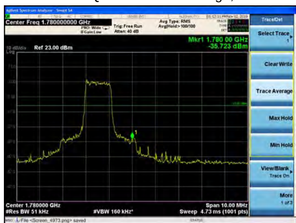
LTE Band 66 QPSK 20MHz CH-High, 1 RB
