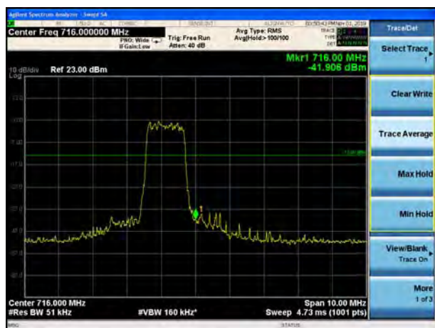
LTE Band 12 QPSK 5MHz CH-High, 1 RB
