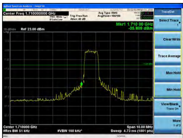
LTE Band 4 16QAM 5MHz CH-Low, 100%RB
