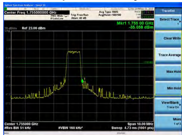
LTE Band 4 16QAM 3MHz CH-High, 1 RB
