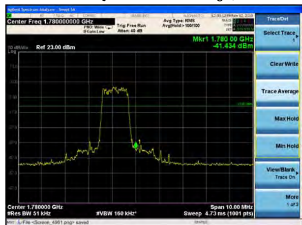
LTE Band 66 QPSK 5MHz CH-High, 1 RB
