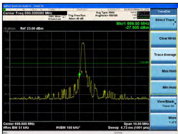
LTE Band 12 16QAM 1.4MHz CH-Low, 1 RB
