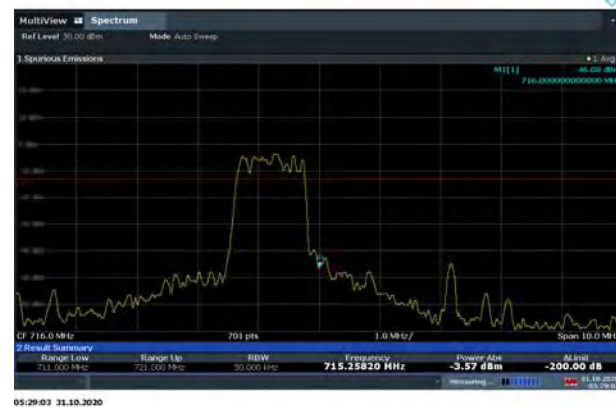
LTE Band 85 QPSK 5MHz CH-High, 100%RB
