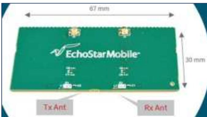
About terrestrial LoRa sub-GHz bands in US915 spectrum, there are already a lot of antennas available in the market and choosing the antenna is part of design done by device Makers. The maximum allowed antenna gain is 10 dBi.
