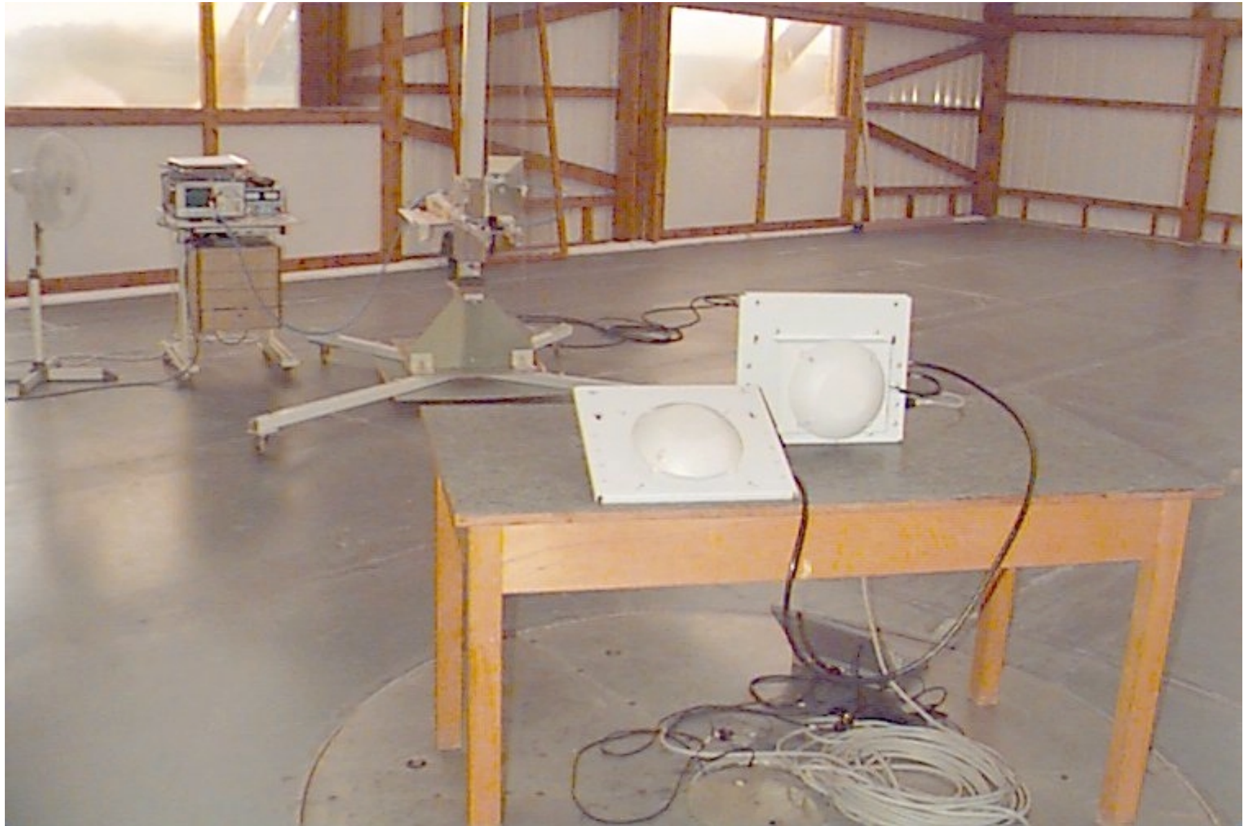
Radiated emission measurements at OATS, above 1 GHz
