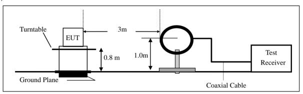
(b) For radiated emissions from 30MHz to 1000MHz
