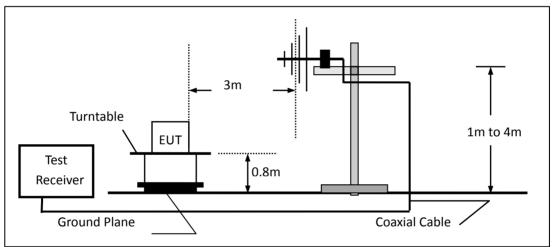
(c) For radiated emissions above 1000MHz
