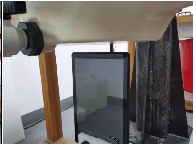
Right Side of EUT with 1.9cm Gap
