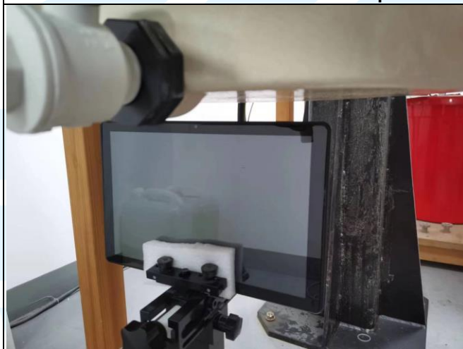
Top Side of EUT with 1.9cm Gap
