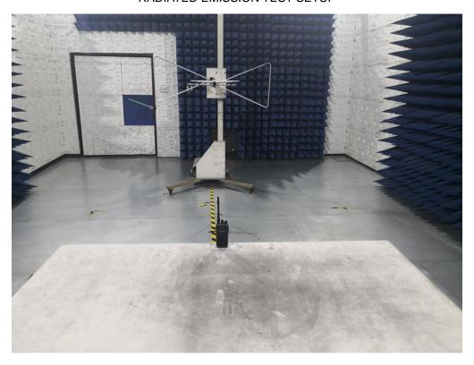
RADIATED EMISSION ABOVE 1G TEST SETUP
