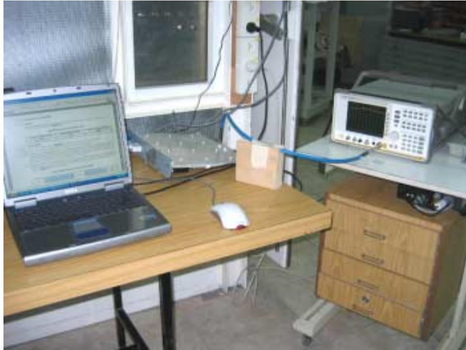
Photograph No.7 BSR peak spectral density test setup
