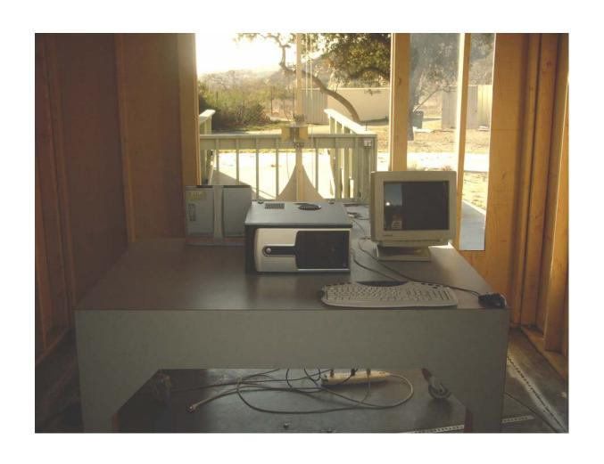
Radiated Emissions Measurement (Front View) Setup
