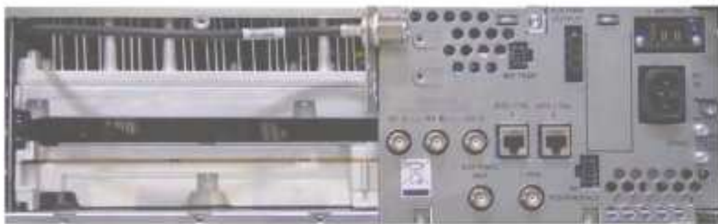
Figure 103: GTR 8000 Base Radio Showing Connections to Backplane Through Backplane Cover
