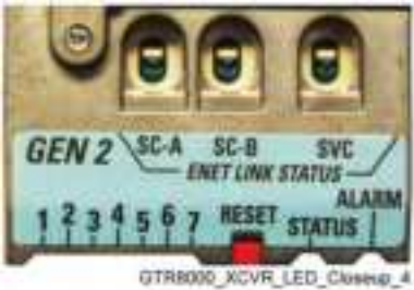
Figure 7: Transceiver RESET Switch (viewable through the drop-down door)
