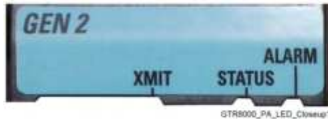
Figure 117: Power Amplifier LEDs, viewable through a drop-down door
