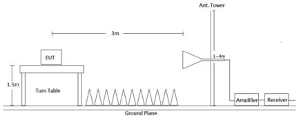
Radiated emission tests were performed in the 3 meters chamber test site, using the setup accordance with the ANSI C63.10-2013. The specification used was the FCC Part 15.209 and FCC 15.407 Limits.
