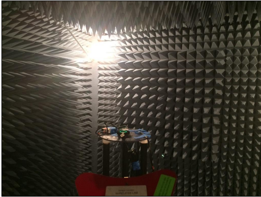
Photograph 3. Radiated Emissions, Test Setup, Above 1 GHz
