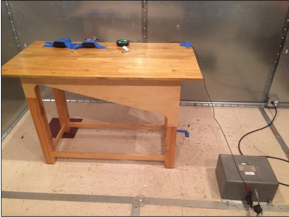
Photograph 1. Conducted Emissions, 15.207, Test Setup
