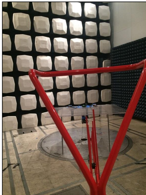
Photograph 2. Radiated Emissions, Test Setup, Below 1 GHz
