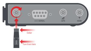
Please refer to the Device overview section for the antenna socket layout. If you have purchased a GPS antenna, remove the socket cap from the GPS antenna socket and attach the antenna to the socket in the same manner.
