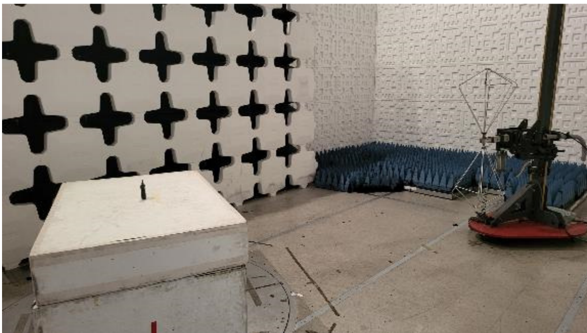
Figure 3. Radiated Emissions Test Setup, 30 MHz to 200 MHz, 0.5-mile (STD00-17811)
