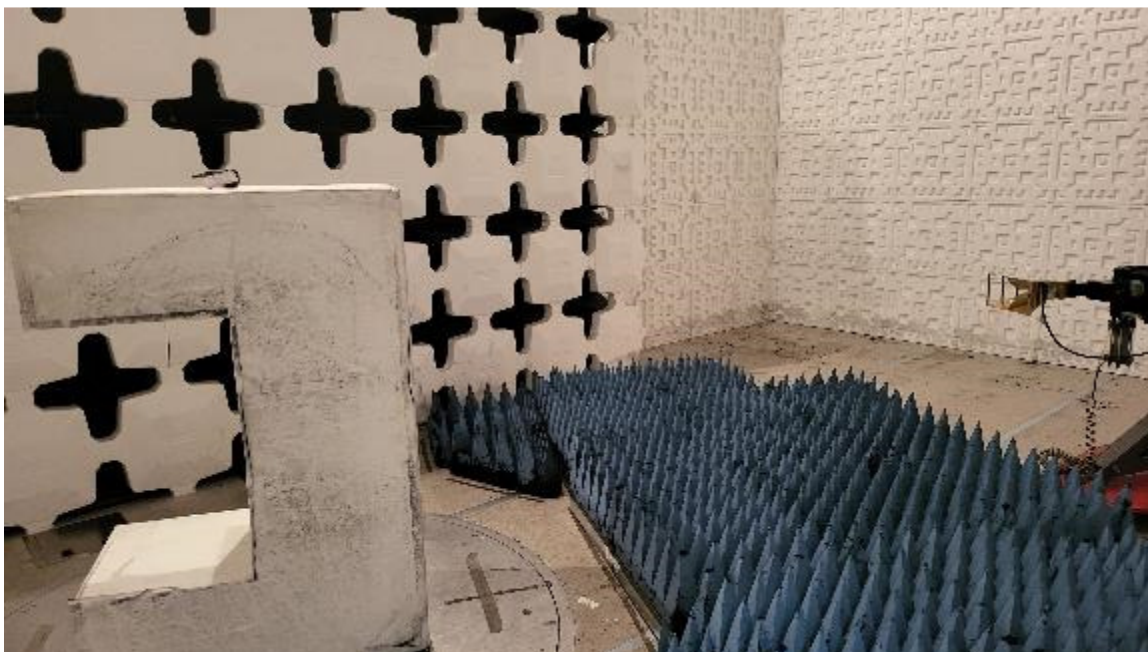
Figure 5. Radiated Emission Test Setup, above 1 GHz, 0.5-mile (STD00-17811)
