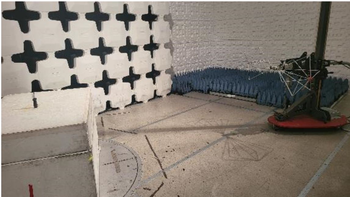
Figure 3. Radiated Emissions Test Setup, 30 MHz to 200 MHz, 1.0-mile (STD00-17812)
