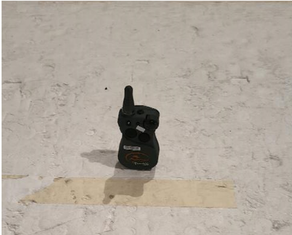
Figure 7. Radiated Emissions Test Setup, 0.5-mile (STD00-17811)
