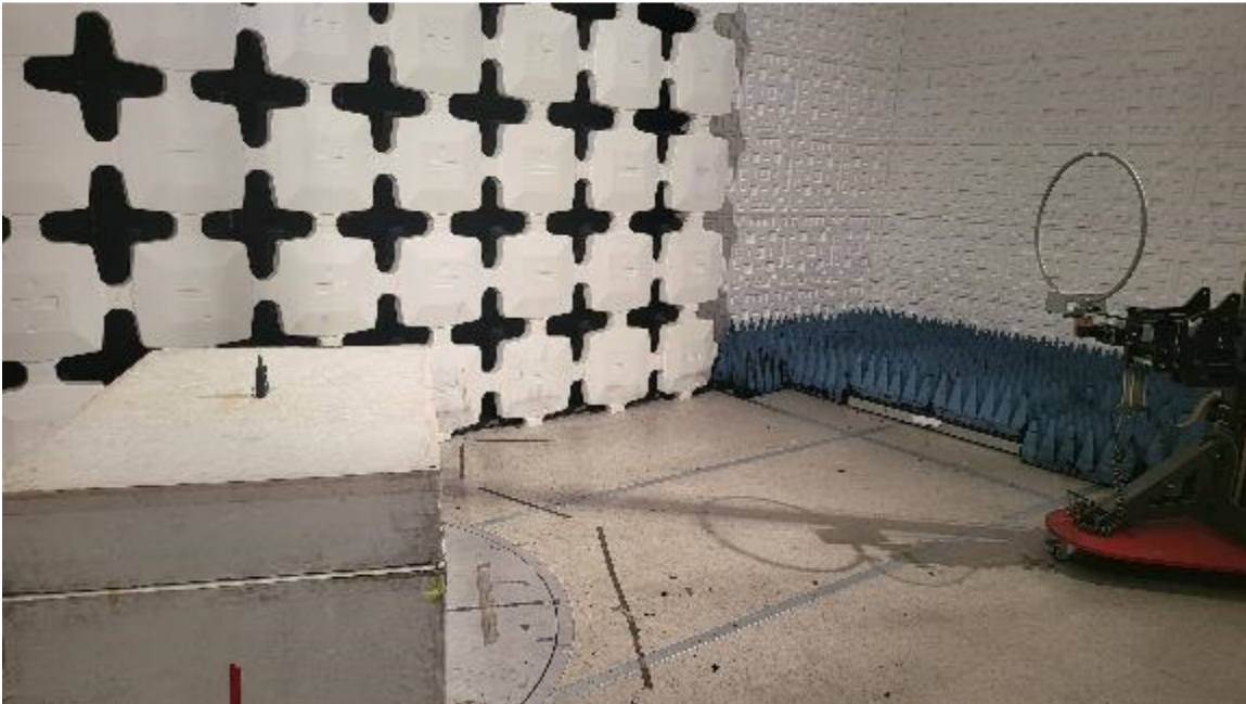
Figure 2. Radiated Emissions Test Setup, .15 MHz to 300 MHz, 0.5-mile (STD00-17811)
