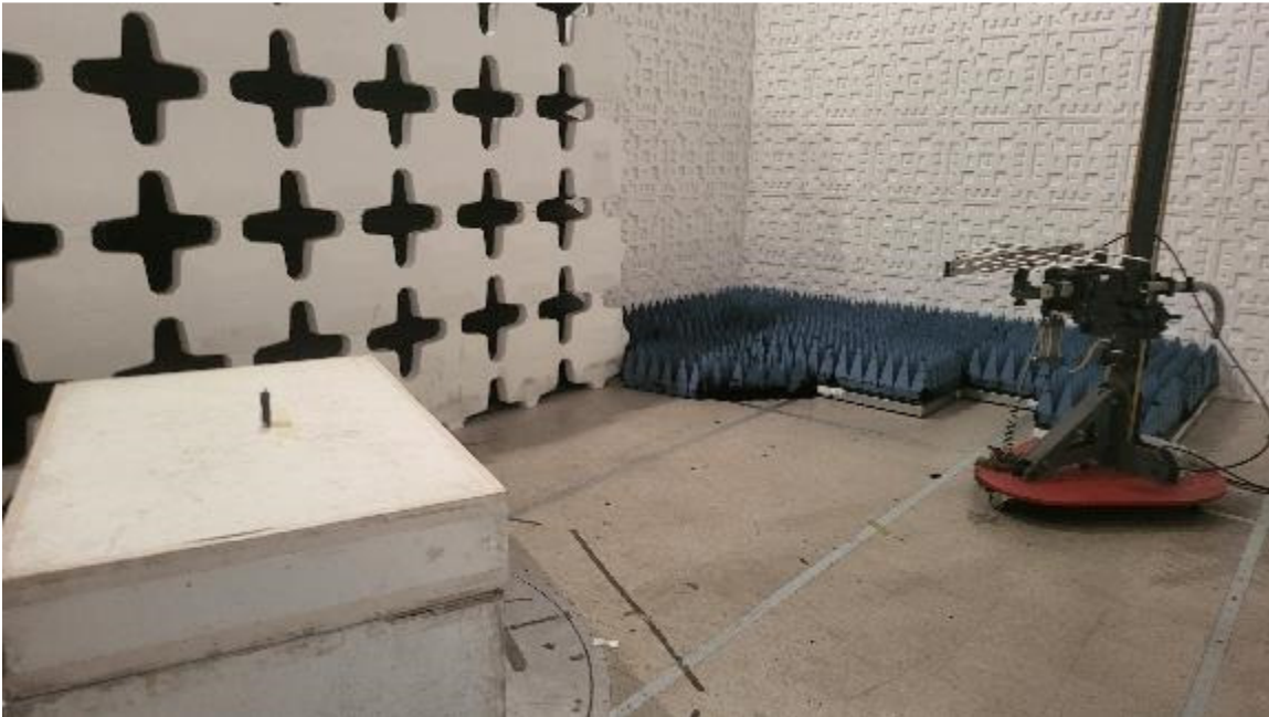
Figure 4. Radiated Emissions Test Setup, 200 MHz to 1GHz, 0.5-mile (STD00-17811)
