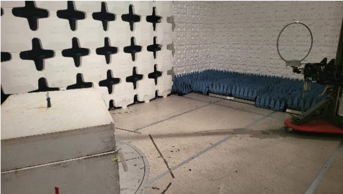
Figure 2. Radiated Emissions Test Setup, .15 MHz to 300 MHz, 1.0-mile (STD00-17812)
