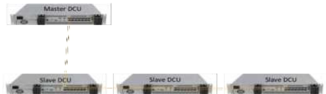
Figure 11. DCU Daisy Connection
