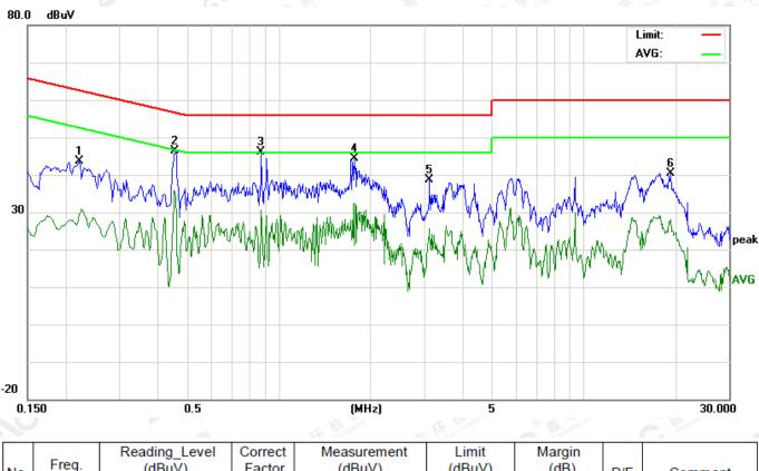
Line Conducted Emission Test Line -N
