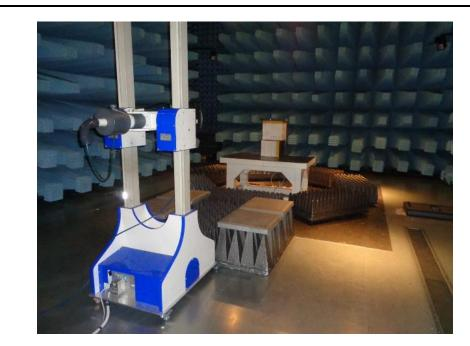
1.2 Radiated emissions set-up for frequencies above 1 GHz up to 18 GHz
