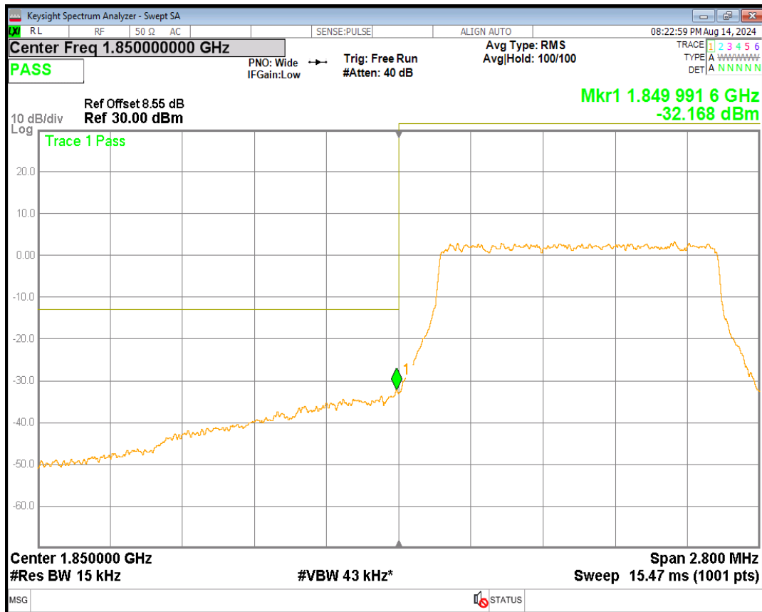
Band25 16QAM BW=1.4MHz Channel=26683 RB Size=6 Position=#0
